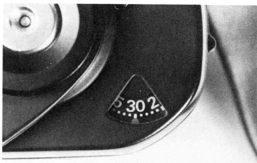
The frame counter of the Nikon F3 is located to the right of the film advance lever.
